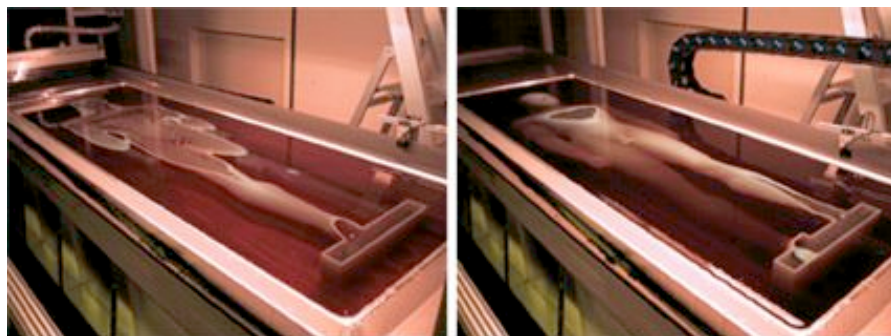
Figure 14 - The statue at 24hr and 86hr build times
